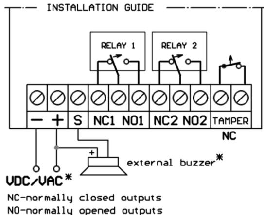
**IMPORTANT! Output S must not** be directly connected to (+) pole of power supply (see schema).
