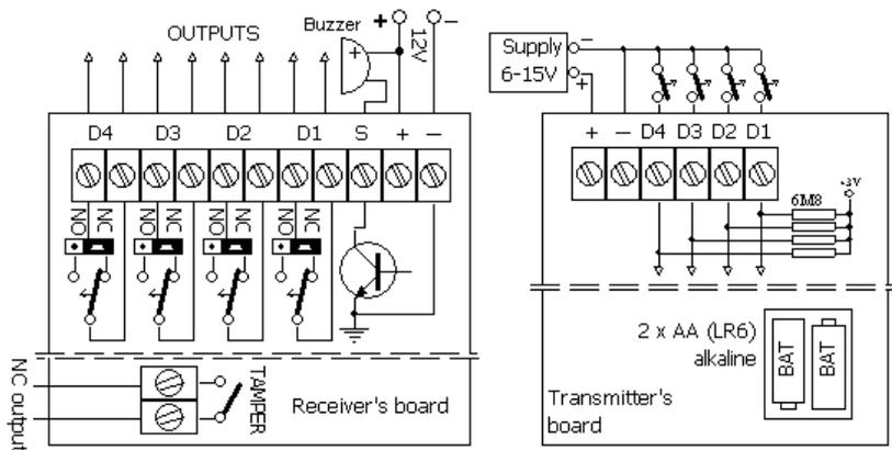
The RP501 transmitter may be either powered by 12VDC supply screwed to +/- connectors or, by 3V (2x AA) battery or, by both power sources simultaneously.
